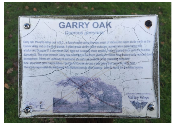
Illustration 8: Faded and cracked plant information sign
